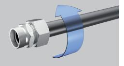
**4.4** Tighten up the coupling by turning the BV-10 union nut by approx. **3/4 – 1 full turns.**
