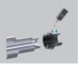
**3.4** Push the tube, with the BV-10 union nut and clamping ring on it, from the outside into the hole of the clamping jaws until it is centred on the BV-10 flared cone.
