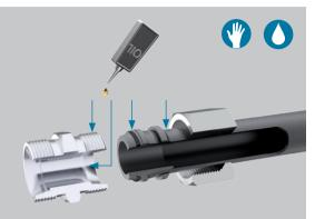
**4.2** Insert the pre-assembled tube end into the cone of the coupling connecting piece at a straight angle.
