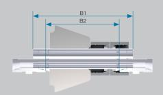
Minimum lengths for clamping in curved tubes (R  $\geq$  3x Tube OD).
